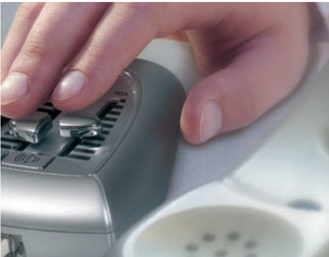
The Inline telephone amplifier PL-51 also has additional amplification. Keeping the amplifier button pressed doubles the set volume.
