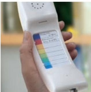
Thanks to embedding the speed dial reference list in the bottom part of the receiver, the user can bring the list close to his eyes without having to bend down to the phone.
